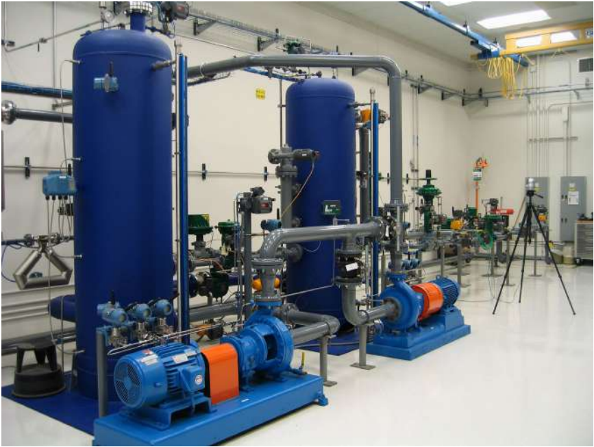
Figure 2.2 Performance Test Loop
