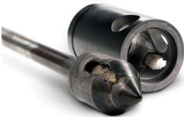
Figure 5.9 Typical Appearance of Cavitation Damage
