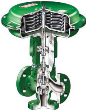
Figure 3.6 Three-Way Globe Valve
