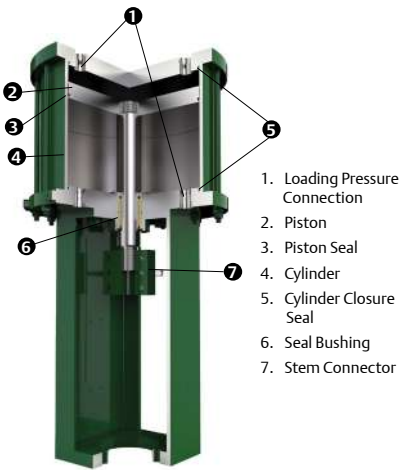
Figure 1.10 Piston-Type Actuator
