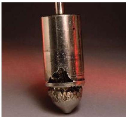
Figure 5.8 Typical Appearance of Flashing Damage
