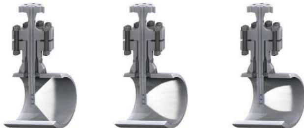
Figure 7.3 Desuperheater Spray Penetration
