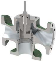
Figure 1.8 Three-Way Globe Valve
