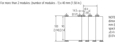
NOTE: All dimensions are in mm (inches). Hole spacing tolerance: ±0.4 mm (0.016 in.).
