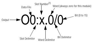
(1) I/O located on the controller (embedded I/O) is slot 0. I/O added to the controller (expansion I/O) begins with slot 1.
