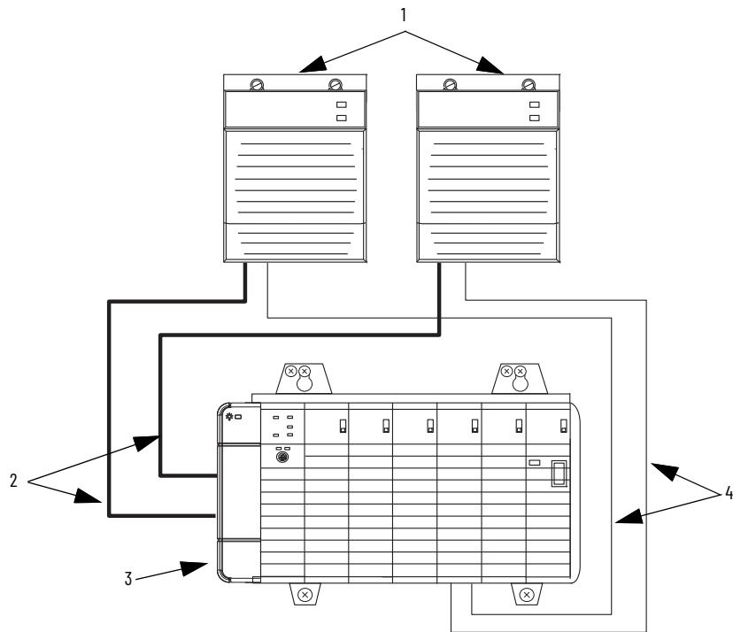
**IMPORTANT** The ControlLogix redundant power supply system is designed to account for operational anomalies in only the power supply. The chassis adapter and power supply cables are excluded.
