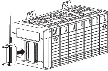
2. Connect the female end of the power cable to the redundant power supply.
